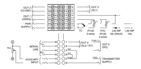
(\*) COM is on terminal 7 for output OUT4, continuous-type (W1). COM is on terminal 11 for output OUT4, relay- or logic-type
