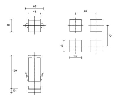
Dimensions: 48x48mm (1/16DIN) depth 129mm
